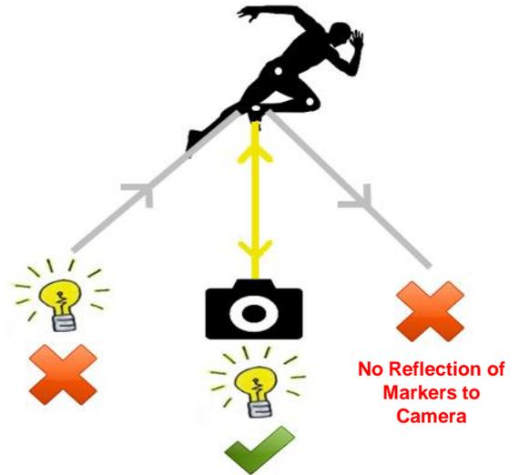
By placing the lighting on a separate tripod you **MUST** position the light source directly behind the camera. Quintic High Speed Cameras and lighting options can be attached directly to the same plate, ensuring that the light source is being emitted in the same direction that the camera lens is pointing.
