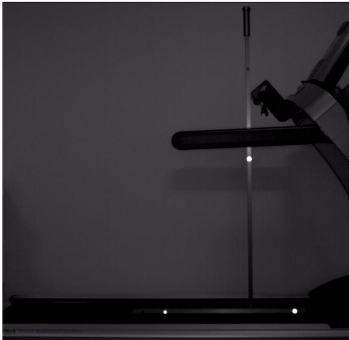
The calibration tool should be large enough to reduce the effect of errors when digitising points. You can imagine if you were trying to calibrate using a tool only a few cm's long, the slightest inaccuracy when calibrating these points would be scaled up to cause large inaccuracies over longer distances.
