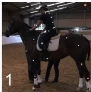
1, horse fitted with IMU's and motion capture markers; 2, one stirrup shortened by 5 cm; 3, rider fitted with motion capture markers
