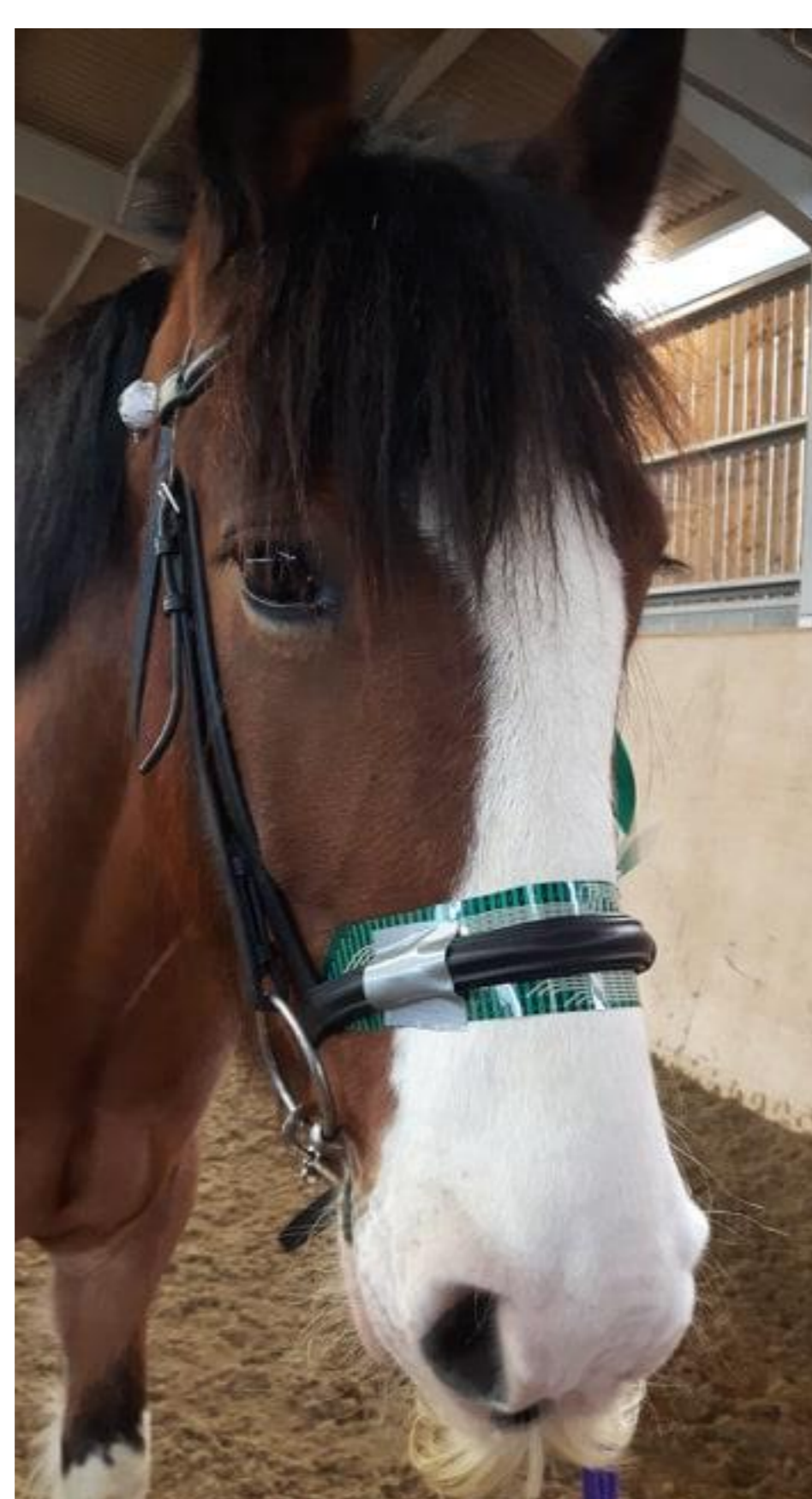
Set up of pressure sensor (F-Scan)
