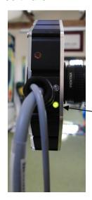
Check the lights on the back of the highspeed camera are flashing to ensure it is connected and powered properly.
