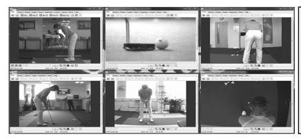
Many Quintic High-Speed Cameras allow video capture of up to 1000 still frames per second (fps) at certain image dimensions, capable of capturing even the fastest human movements. Quintic Software allows for up to six Quintic High Speed videos to be imported and analysed live.
