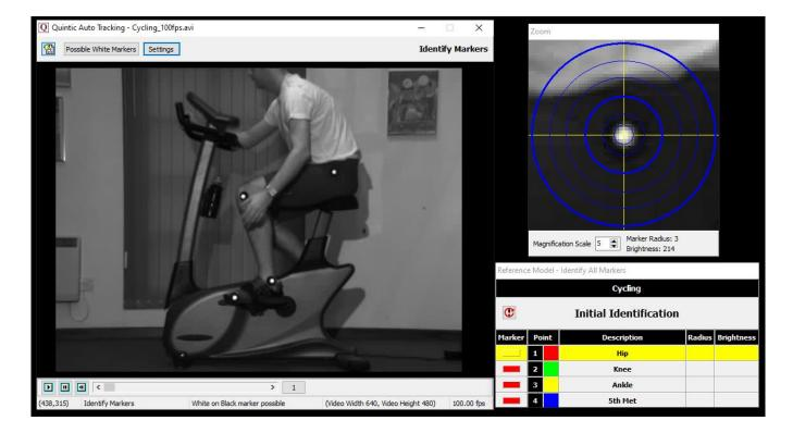
As the cursor moves across the screen, the magnification window shows a larger version of the area under the cursor. The magnification window allows the user to pinpoint the exact marker locations. This must be done in the correct order. The reference template illustrates the order of marker identification.
