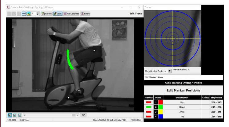
This will bring up all of the digitisation points for every frame that has been digitised, one point at a time. The point that is currently active will be displayed in green, so for the example above, the hip point is displayed. All the other points in the marker set will be highlighted in red within the Edit Marker Positions box.
